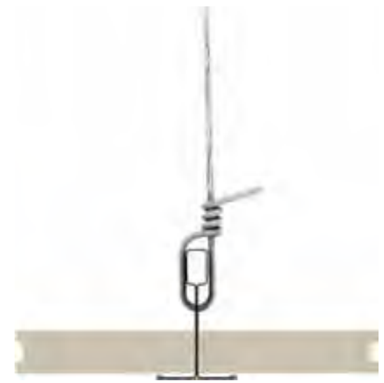
Figure 5 Exposed tee grid
