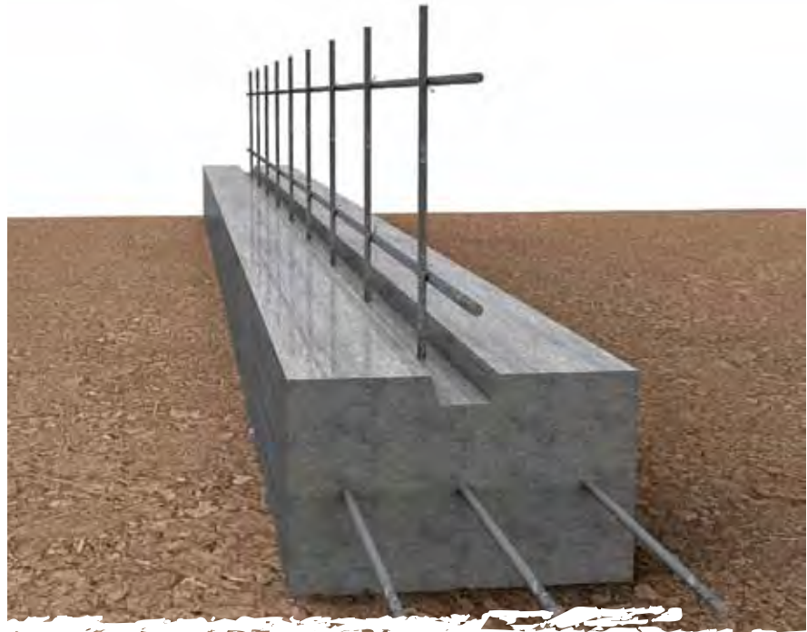
Figure 15 Embedded vertical reinforcing bar
